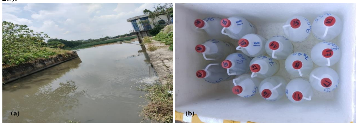
Figure 2. (a) Ba Bo canal – Binh Duong, where waste containing microplastics from wastewater treatment plants is discharged; (b) Water samples are ready to be sent to the microplastic analysis laboratory.
