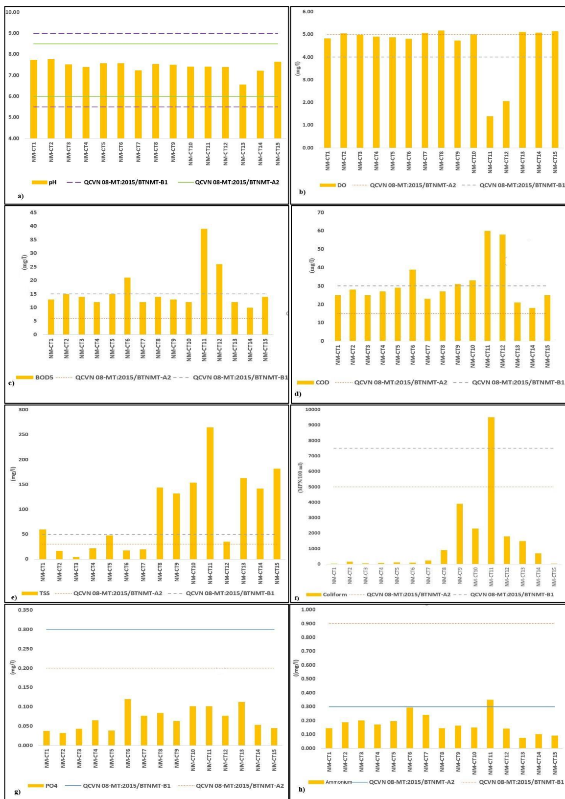
Figure 6. Measured values of water quality parameters at sampling sites on Ca Ty River: (a) pH parameter; (b) DO parameter; (c) BOD 5 parameter; (d) COD parameter; (e) TSS parameter; (f) Coliform parameter; (g) Phosphate parameter; (h) Ammonium parameter.
